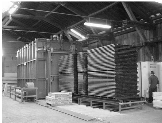
Figure 1 : HTT Plant – NOW Process (retification)
