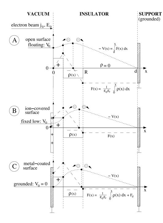
Fig. 1 Plus-minus charge distribution  $\rho(x)$  beneath the surface and the respective electrical field F(x) and potential V(x) distributions in a dielectric on a conducting support with an open surface: A; an ion-covered surface: B; and a metal covered and grounded surface: C.
