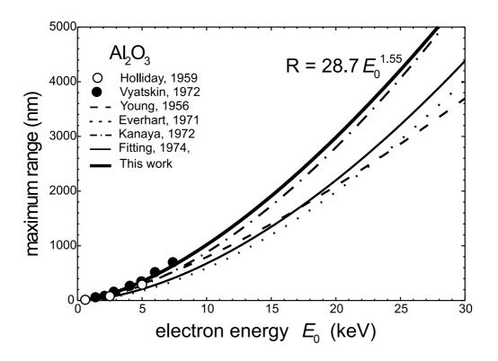
Fig. 2 Measurements (Refs. 31, 32) and experimental fits (Refs. 33 - 36) of the maximum range  $R(E_0)$  of electrons with initial energy  $E_0$  in amorphous Al<sub>2</sub>O<sub>3</sub>.
