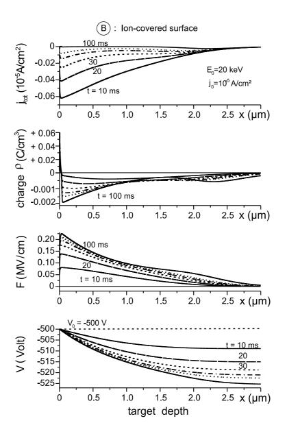
Fig. 13 Current  $j_{tot}(x)$ , charge  $\rho(x)$ , electric field F(x), and potential V(x) depth distributions beneath the positive-ion-covered surface ( $V_0 = -500$  Volt) of alumina in dependence on irradiation time t; electron beam energy  $E_0 = 20$  keV and current density  $j_0 = 10^{-5}$  A/cm<sup>2</sup>.
