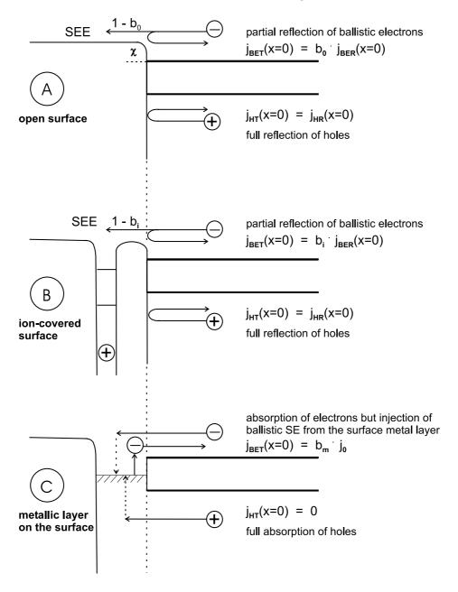
Fig. 12 Surface reflection and/or absorption of electrons and holes at: A: open surface;B: positive-ion-covered surface, and C: metallized and grounded surface.
