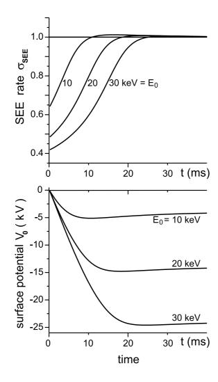
Fig. 9 Secondary electron emission rate  $\sigma$  and surface potential  $V_0$  of bulk alumina targets as function of irradiation time t for different electron beam energies
