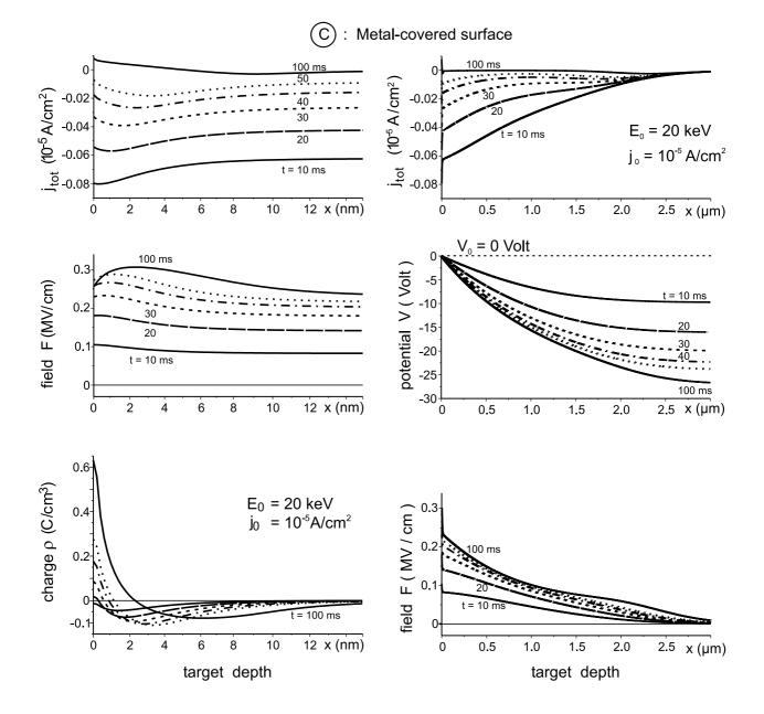
Fig. 14 Current  $j_{tot}(x)$ , charge  $\rho(x)$ , electric field F(x), and potential V(x) depth distributions beneath the positive metal-covered and grounded surface  $(V_0 = 0)$  in dependence on irradiation time t, zoomed in nm scale (left) and presented in  $\mu$ m scale (right); electron beam energy  $E_0 = 20$  keV and current density  $j_0 = 10^{-5}$  A/cm<sup>2</sup>.
