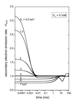
Fig. 10 Secondary electron emission rate  $\sigma_{\text{SEE}} = \eta + \delta$  in dependence on irradiation time for different PE energies  $E_0 = (0.5 - 7)$  keV in the transition region  $\sigma \stackrel{\geq}{<} 1$ ;  $j_0 = 10^{-5} \text{ A/cm}^2$ .
