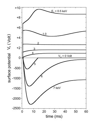
Fig. 11 Surface potential  $V_0$  in dependence on irradiation time for different PE energies  $E_0 = (0.5 - 7)$  keV in the transition region  $\sigma \stackrel{\geq}{\leq} 1$ ;  $j_0 = 10^{-5}$  A/cm<sup>2</sup>.
