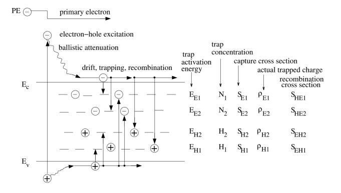
Fig. 5 Scheme of the flight-drift model including the ballistic flight and attenuation followed by drift, trapping, and recombination of electrons and holes.
