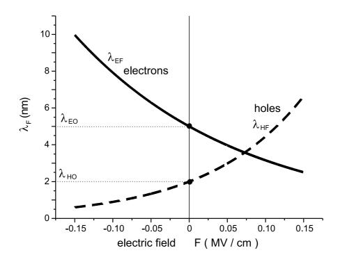
Fig. 4 Mean attenuation lenghts of electrons  $\lambda_{\rm EF}$  and holes  $\lambda_{\rm HF}$  in Al<sub>2</sub>O<sub>3</sub> as a function of the electric field *F*, according to Eq. (11).
