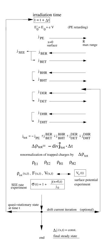
Fig. 7 Computation scheme of the selfconsistent charging in insulating samples.
