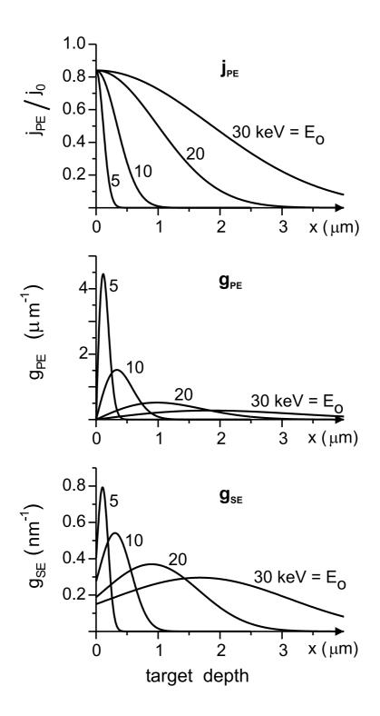
Fig. 3 Current  $j_{\text{PE}}(x)$  of primary electrons with initial energy  $E_0$  into Al<sub>2</sub>O<sub>3</sub>, their deposition (absorption) function  $g_{\text{PE}}(x)$ , and their secondary electron generation  $g_{\text{SE}}(x)$ , according to Eqs. (4) - (9), respectively.
