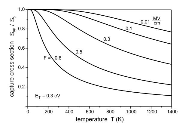
Fig. 6 Poole-Frenkel-modified capture cross sections  $S_{\rm PF}$  according to Eq. (25) of a shallow trap with thermal activation energy  $E_T = 0.3 \,\mathrm{eV}$  in dependence on temperature Tand electric field F.
