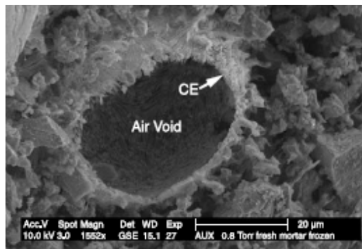
Figure 2: Fracture surface of a previously shock-frozen fresh mortar with an air void surface covered with cellulose ether (ESEM in situ cryo-experiment) [9].
