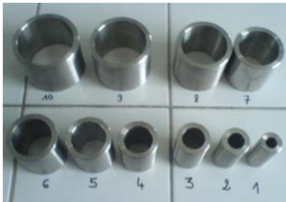
Figure 5: Test devices to measure mortar consistency.
