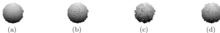
Fig. 3. Representation of aggregates with a spherical convex hull and different filling ratio: (a) full filling, (b) hollow filling, (c) random filling at 50%, (d) random filling at 75%
