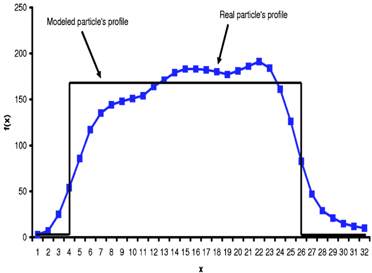
Figure 4: Real and modeled particle 1-D profile: blue squares indicate the profile of a real “perfect” (not blurred) particle image; in black, the corresponding squared modeled profile. (Color online only).
