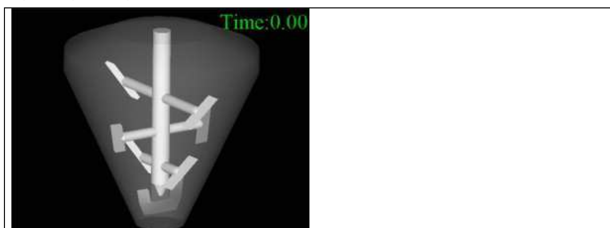
Figure 4: The geometry of the modeled Cyclomix.
