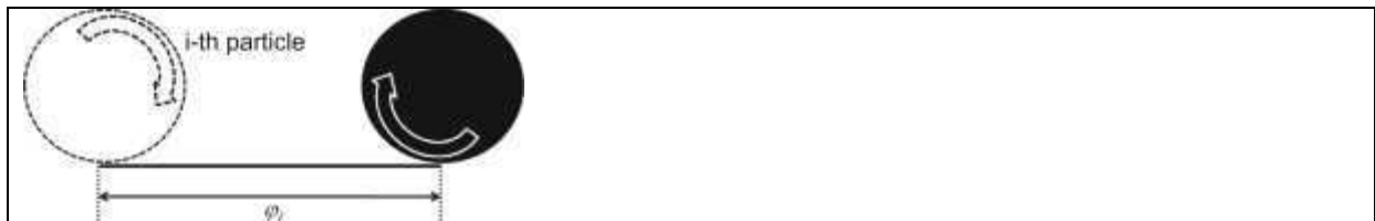
Figure 5: Definition of rotational distance of the i -th particle.
