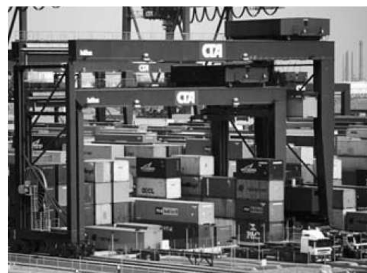
Figure 1.8: Yard run with rail mounted gantry cranes
