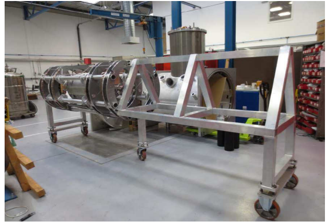
Figure 3: Loading/unloading the cryostat with an aluminum frame.
