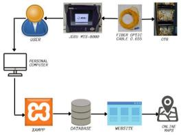
Figure 1. Block Diagram
