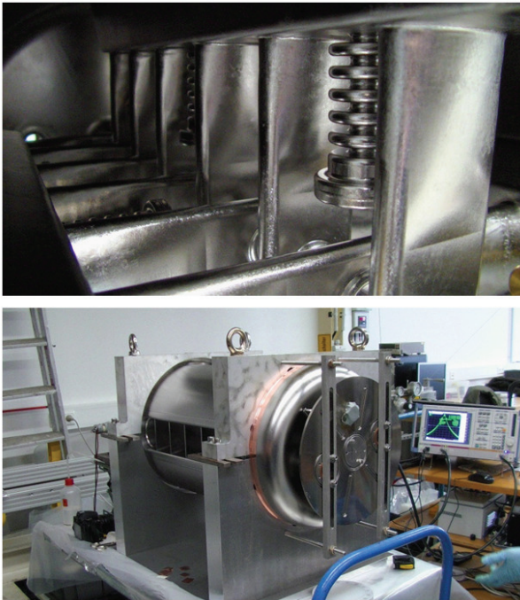
Figure 3: Current status of the cavity with temporarily attached end caps (top), measurement setup (bottom).
