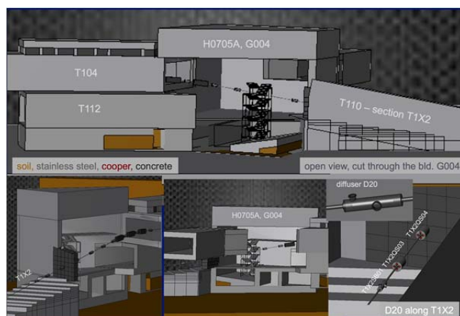
Figure 1: FLUKA geometry of bld. G004 with the diffusor D20 along the sloped beam line T1X2.
