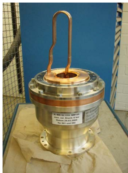
Figure 2: Prototype of the RF coupler for the CH-cavities of the pLINAC
