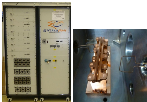
Figure 2: Amplifier (left) and RFQ test cavity structure.
