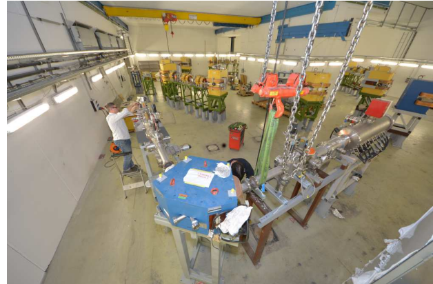
Figure 1: Photograph of the situation in the CRYRING cave end of 2014. In the foreground the local injector has been setup and is being aligned. In the background visible is the ring structure with its dipoles and the magnetic sections with quadrupole and sextupole magnets.
