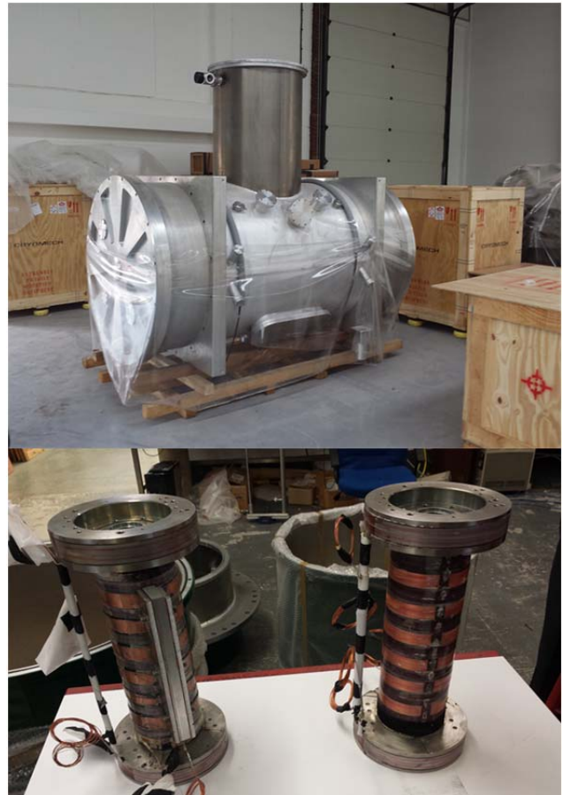
Figure 2: The cryostat and the two sc solenoids are ready for assembling at Cryogenic Ltd, London.
