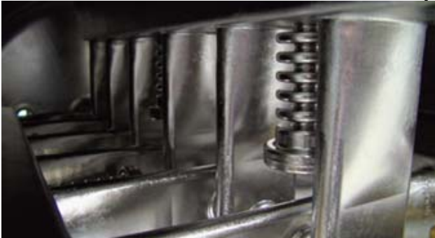
Figure 1: The inner structure of the CH-cavity.
