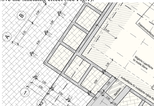
Figure 1: 2011 layout of south-east part of the building G50 with enclosed soil packs on the outside wall.
