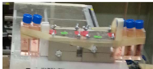
Figure 3: Example of experimental device used for verification of microenvironment adapted treatment planning: biological phantom composed by normoxic cells (tissue culture flasks) and cells at different oxygenation conditions (hypoxic chambers).
