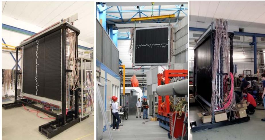
Figure 1: The first NeuLAND double-plane in its frame in Cave C (left), NeuLAND double-plane no. 4 on its way to Cave C (middle, photo: G. Otto) and the demonstrator support frame after insertion of the fourth double-plane (right).
