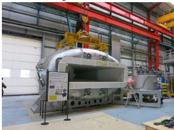
Figure 1: R 3 B Glad magnet during the welding of the cryostat at CEA/Saclay
