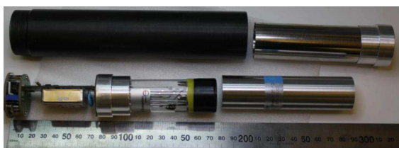
Figure 1: The components of the LaBr 3 detector.
