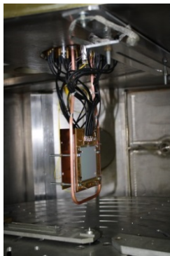
Figure 1: Si strip detectors inside the scattering chamber of ACCULINNA separator.
