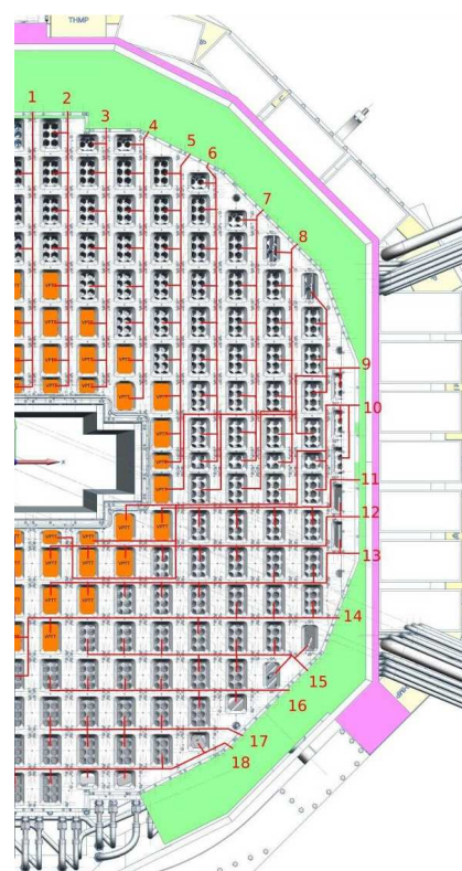
Figure 1: Routing scheme of the backplate part for one half of the forward endcap.
