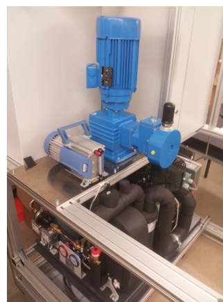
Figure 2: Vacuum pump set-up with condensing unit.
