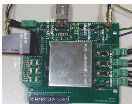
Figure 1: Test PCB for the STSXYTER ASIC.
