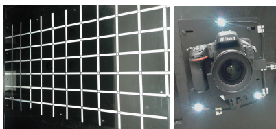
Figure 1: CLAM equipments used in the RICH prototype. Retro-reflective grid, with target dots (left). CLAM camera, surrounded by three LEDs (right).
