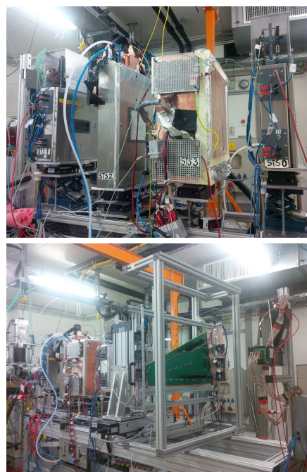
Figure 1: (Top) Telescope with four silicon detector stations. The second to the right operates the irradiated sensors. (Bottom) A full-size prototype GEM sector was installed further downstream comprising a triple-GEM foil stack.
