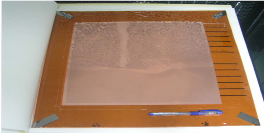
Figure 3.36: One single layer 30\text{cm}\times 30\text{cm} GEM detector
