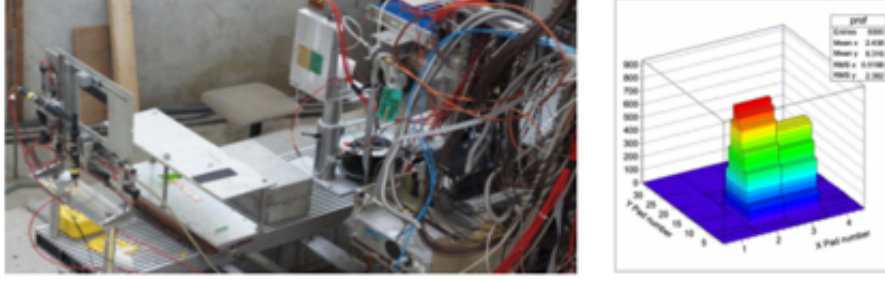
Figure B.1: One of the chambers located at the CERN T-10 area (left). An example of the beam profile measured with the chamber is also depicted (right)
