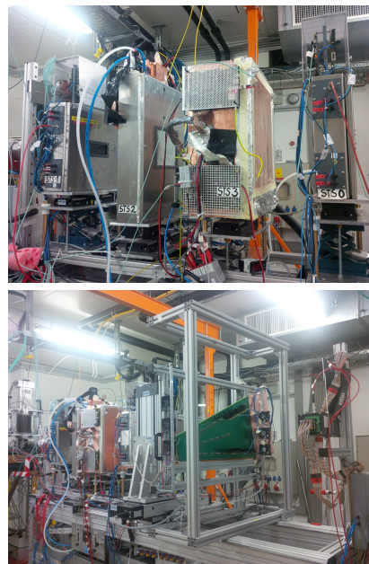
Figure 1: (Top) Telescope with four silicon detector stations. The second to the right operates the irradiated sensors. (Bottom) A full-size prototype GEM sector was installed further downstream comprising a triple-GEM foil stack.
