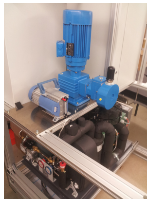
Figure 2: Vacuum pump set-up with condensing unit
