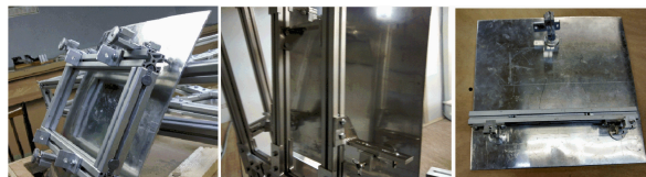
Figure 3: Mounting options for the mirror tiles. Left: base case (aluminum rectangle); middle: 3 independent mounts; right: 2 aluminum bars.
