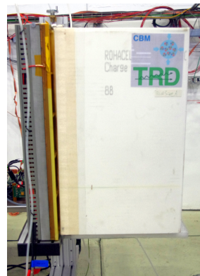
Figure 2: Side view of the real-size TRD prototype in the PS/T9 beam line in 2014 with a mounted full-size foam foil radiator
