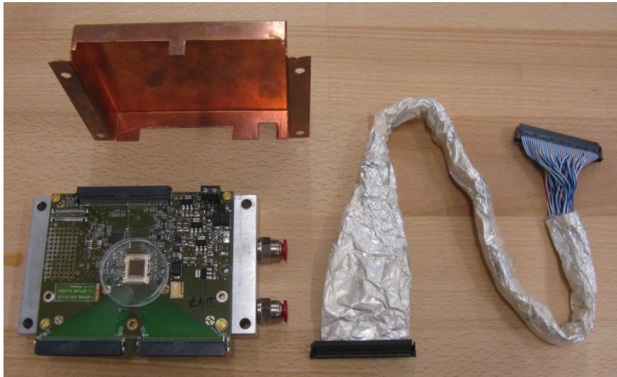
Figure 6.9: n-XYTER based front-end board, a shield for it, and a shielded back-end cable.
