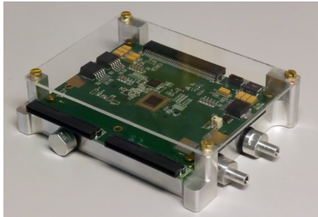
Figure 2.9: General purpose front-end board (FEB), based on n-XYTER chip (board revision D).
