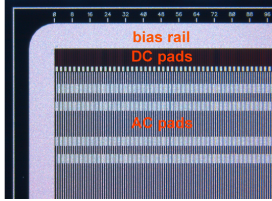
Figure 2.2: Close-up of the n-side of a CBM01 baby sensor. The n-side of the full-size CBM01 sensor, looks similar.
