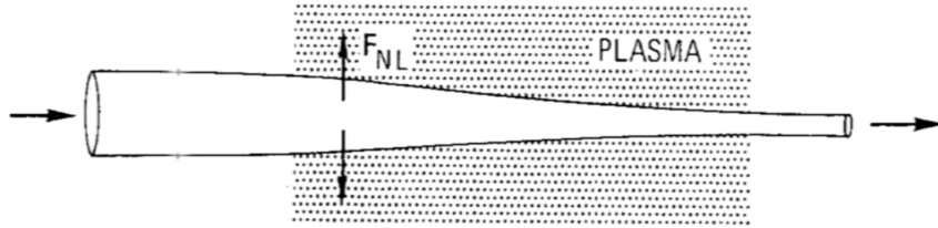
Figure 2.5: Sketch of relativistic self focusing due to the ponderomotive force F_{NL} that pushes the plasma out and thus creating a localized lower plasma frequency \omega_p on the beam axis. This changes also the refraction index and acts as a convex lens that focuses the incident laser beam further. Picture taken from [39].
