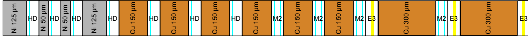
Figure 5.7: Example RCF stack configuration, covering proton energy range from 7 MeV to 38 MeV (left to right).
