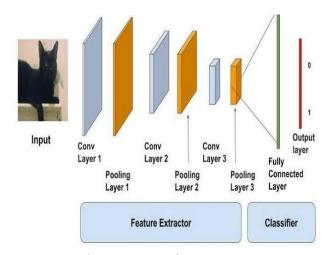
Figure 1: CNN Architecture
