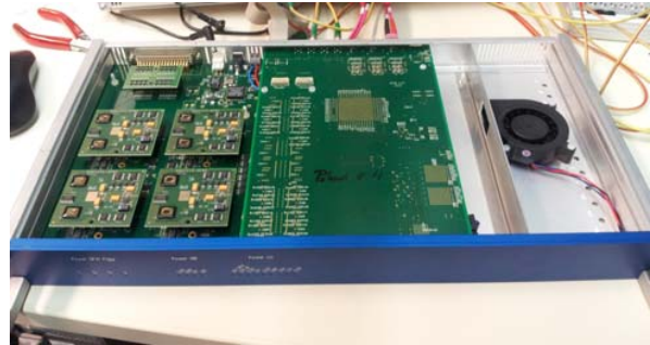
Figure 1: Picture of a 32 channel readout system, including the four QFW units (left side) and the FPGA logic unit (middle). The complete system fits into a 1U 19" rack crate. All connectors are on the back side.
