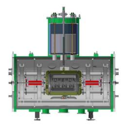
Figure 1: The cw Demonstrator comprising a CH cavity embedded by two solenoids on a support frame.
