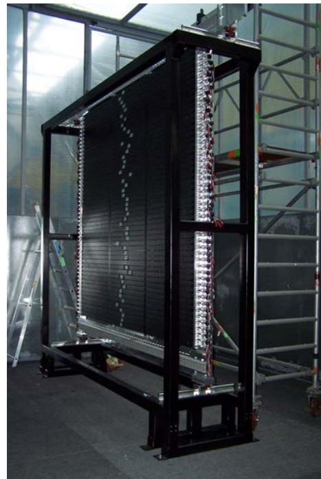
Figure 3: Photograph of the NeuLAND mounting and demonstrator rack together with the first NeuLAND double-plane.
