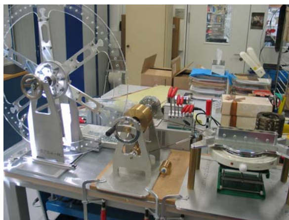
Figure 2: The devices to wind the rings with variable size, thickness and fibre content. The roving comes from the right, goes through a impregnating bath, and is kept on a constant force by a controlled brake before it is wound to the spool (shown on the left).
