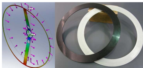
Figure 1: Left: FEM simulation is used to estimate the deformation of the part. Right: small test parts of basalt and glass fibres.
