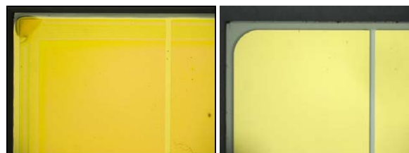
Figure 2: HADES diamond detectors prepared with the Cr+Au metalization, electrodes are processed with the laser lithography. Left: the corner of the diamond plate with the photoresist bead buildup, right: the electrode after etching and the photoresist removal. The feature size (gap between the electrodes) is 80 \mu\text{m} .
