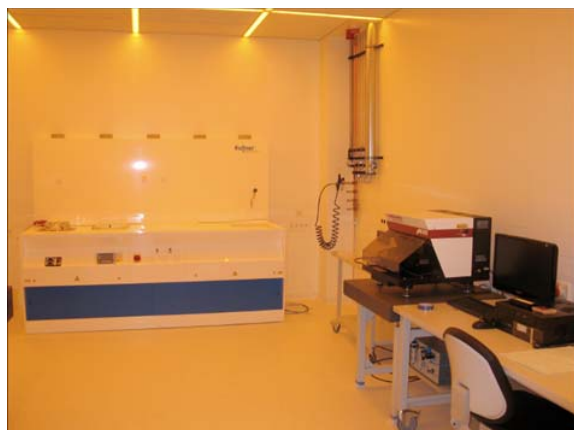
Figure 1: Lithography room in the clean room area of the Detector Laboratory. Working table with the spin coater and the hotplate (left in the photo), and the laser pattern generator with control computer (right).
