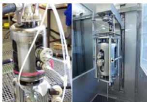
Figure 1: Set-up for BCP (left), Mounting for HPR (right).
