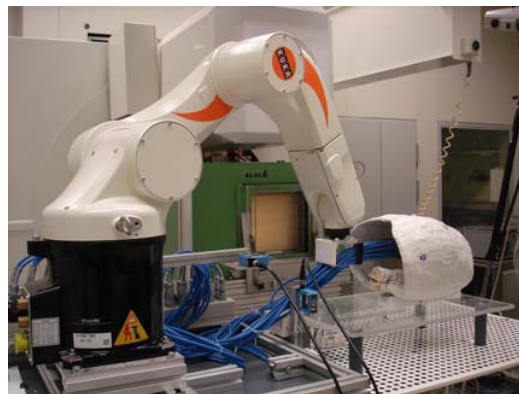
Figure 1: Picture of the Kuka robot holding the PMMA block with ionisation chambers inside the anthropomorphic breathing phantom.
