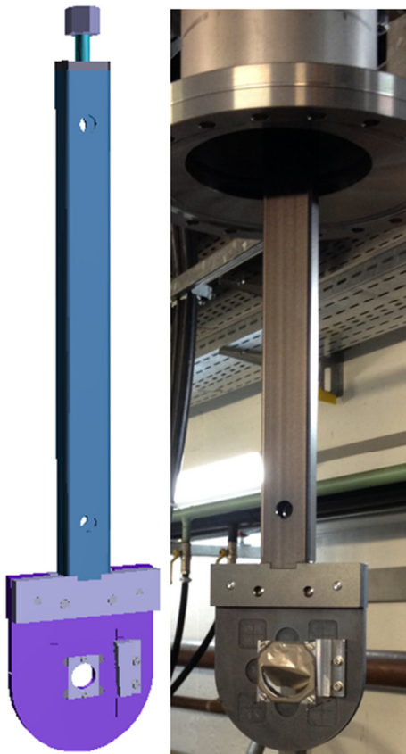
Figure 12: The stripper foil arm installed inside the solenoid is equipped with a polished stainless steel block to reflect the foil image for non-destructive online observation of the foil condition.
