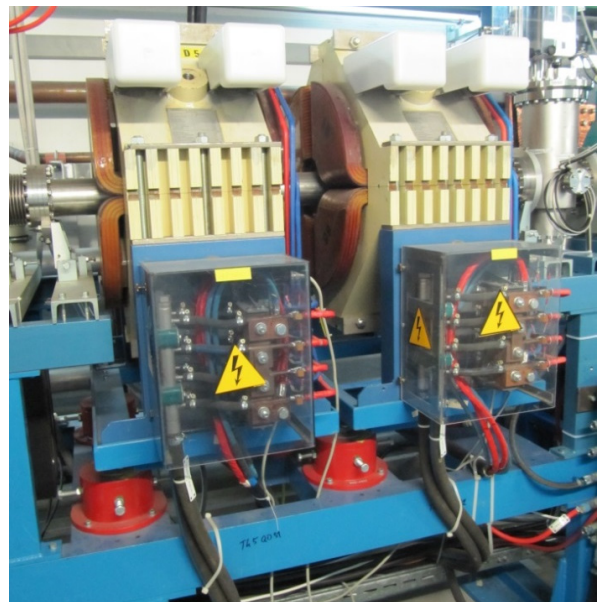
Figure 10: TK5QD5, the already existing quadrupole doublet, together with QD4 it provides a small beam spot and a double-waist on the foil to mitigate emittance growth from scattering during stripping.
