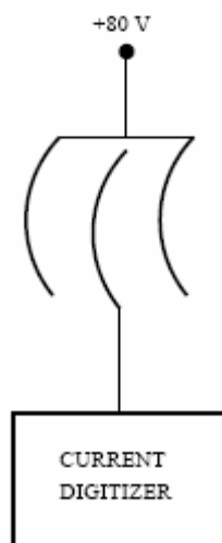
Fig. 2.2. The schematic view of the beam monitor SEETRAM
