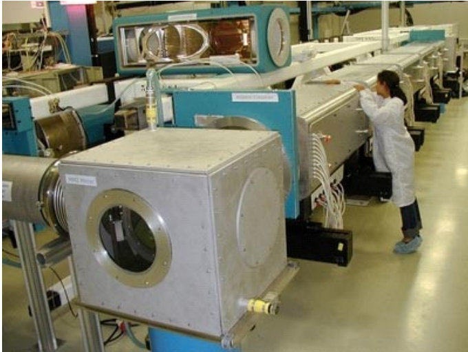
Figure 3: PHELIX 2-pass amplifier section. The beam line is sealed and flushed with nitrogen
