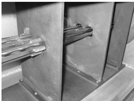
Fig. 2: Photo of the accelerating part of the RFQ, changing to the 3d focus end part. In the background beam line are still the unmodulated electrodes implemented.
