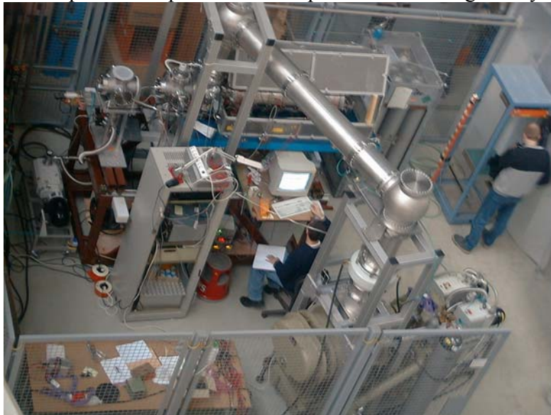
Figure 50: Off-line setup of a high-pressure helium-filled stopping system for relativistic heavy ions. The present gas cell was constructed and assembled in Argonne (ANL) for tests relevant to the RIA and FAIR projects.
