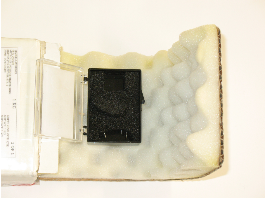
Figure B.3: Transport and storage box with tungsten wires. The tips point into the space that has been cut free from foam plastic.
