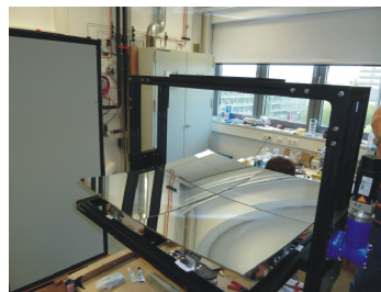
Figure 3: Prototype mirror assembly; the mirrors are already glued to the holders.
