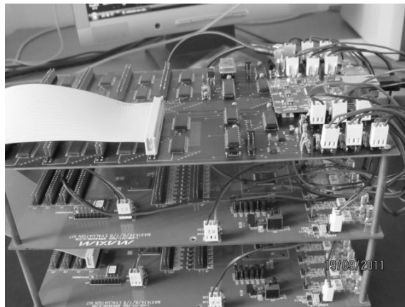
Figure 1: Free running mode acquisition for a high counting rate TRD device
