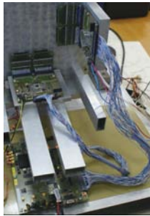
Figure 1: A three-stage GEM detector (back side view) with FEE electronics (based on the nXYTER) at the laboratory test stand
