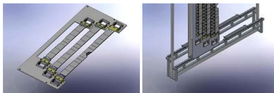
Figure 3: (Left) A block of ladders. (Right) Half-station of a two-station module with two blocks mounted.
