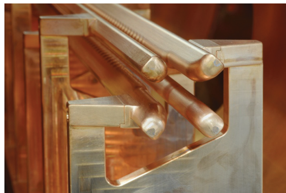
Figure 2: Final assembly inside the RFQ tank.
