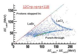
Figure 2: 2D spectrum of the protons from simulation of  ${}^{12}C(p,2p){}^{11}B$  reaction at 400 MeV/u.
