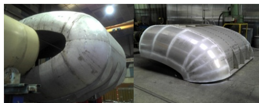
Figure 2: Vacuum vessel and thermal shield panel under construction
