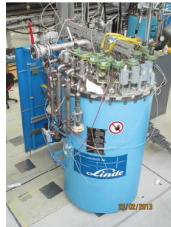
Figure 2: Linde TCF 50 Coldbox.
